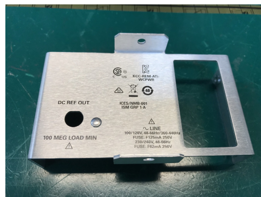
Figure 6-6 11683A-FG new rear panel
