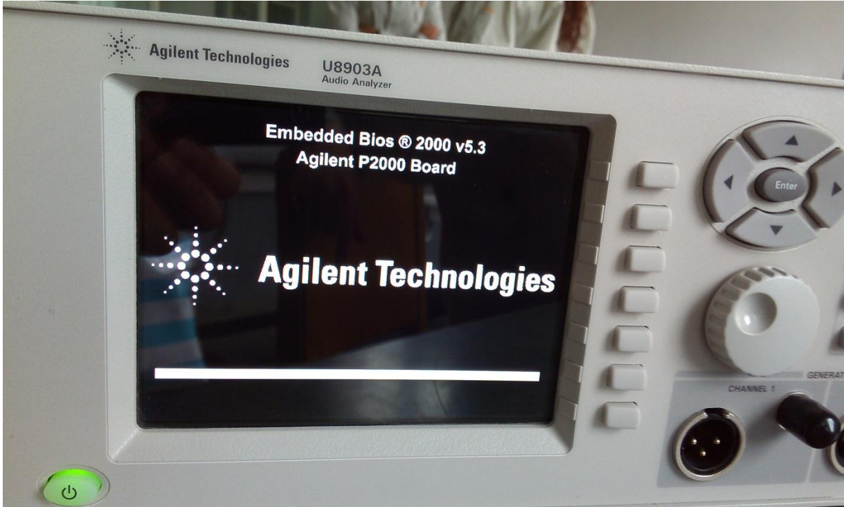
Picture 1 : Picture of unit hang during boot up sequence
