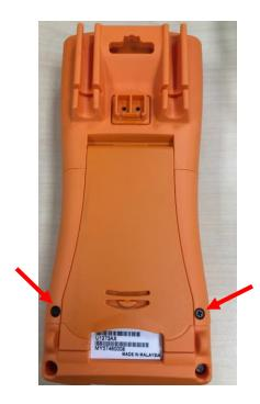
4. Loosen the 4 screws as shown below to remove the bottom cover:
