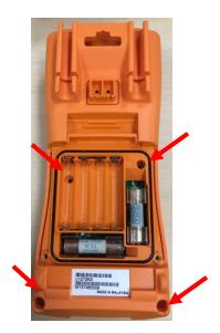
10. Install the battery cover and the two screws to lock the battery cover compartment.
