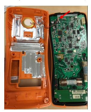
9. Install the back cover and the 4 screws to lock the compartment. Then install batteries.
