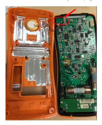
6. To remove the PCA from the top cover, use a flat-head screwdriver and carefully remove the PCA from the latch.
