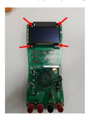
8. Carefully assemble the PCA back to the top casing. Remember to plug in the buzzer wire.
