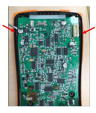
7. Replace OLED display board by unscrewing the 4 screws.
