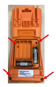
10. Install the battery cover and the two screws to lock the battery cover compartment.
