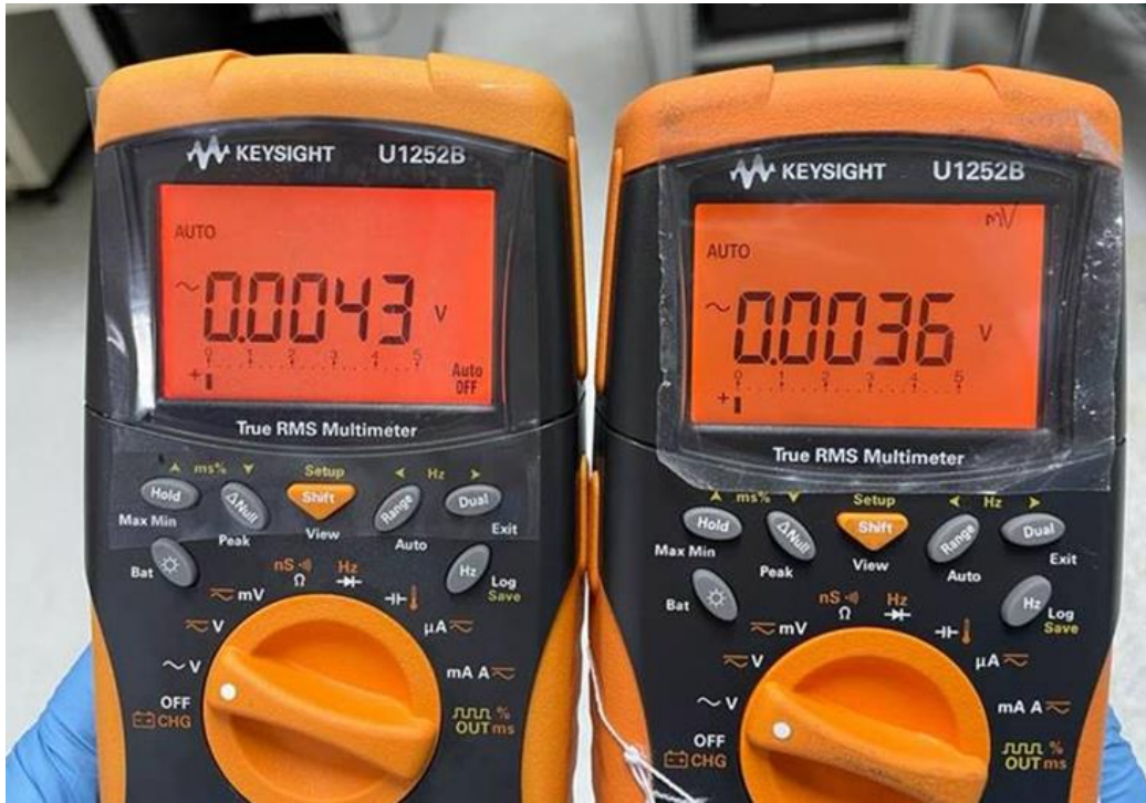
Left: New backlight color (600nm) Right: Original backlight color (598nm)
