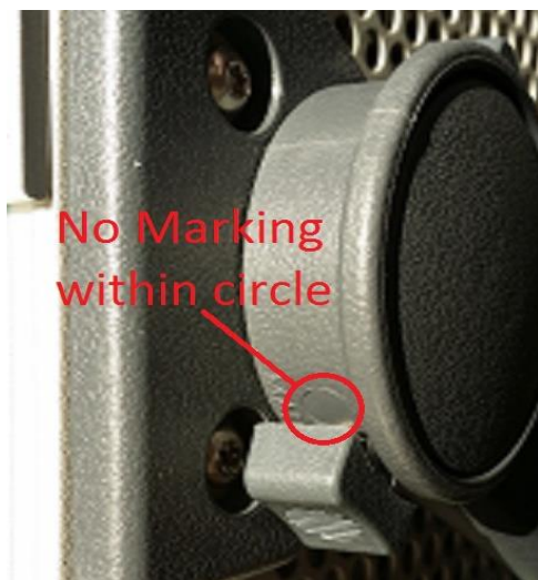
Figure 1. Circle with no markings. This handle should be replaced.
