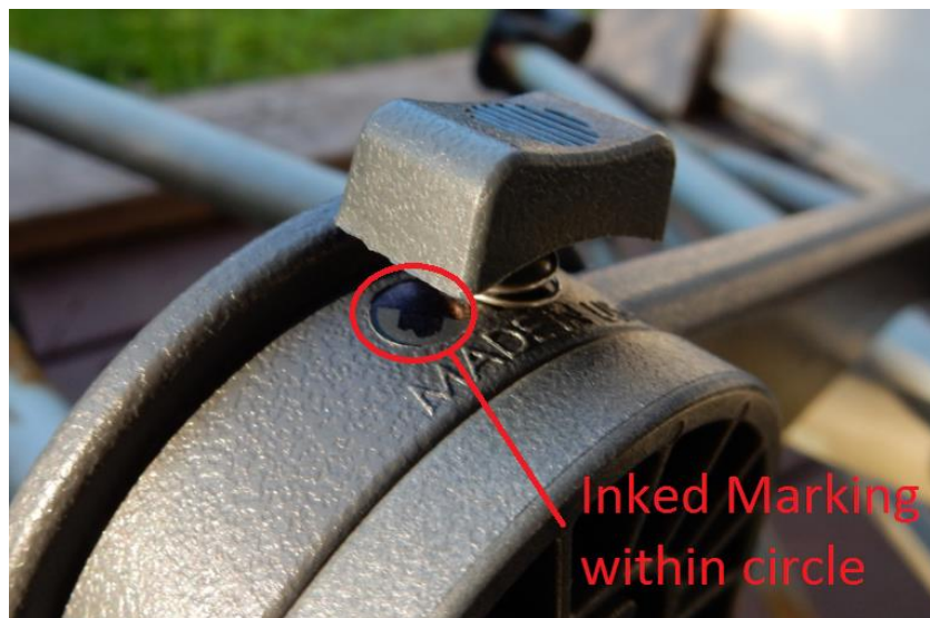
Figure 2. Circle with inked marking. This handle is OK.
