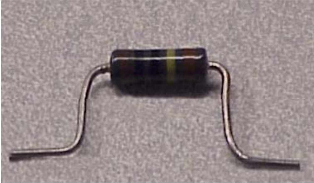
Figure 3. Demonstration of adjusting leads of the 1Mohm bleeder resistor
