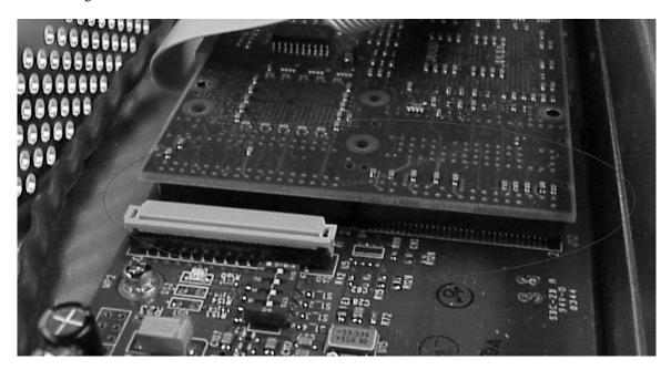
8. Pull up on the top board to see if the two boards are securely fastened together.
