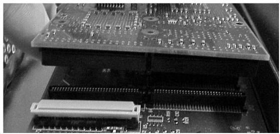
9. Push down on top board until the two boards are securely fastened.
