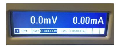
LCD (blue/white display assembly, p/n 2090-1031) has been discontinued by vendor. Replacement assembly (pictured later) is p/n 5067-6532 (amber in color). Difference in color is unfortunate, but cannot be altered.
