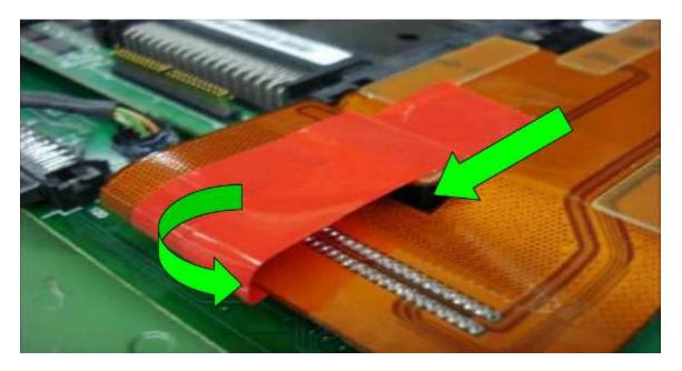
3. Ensure that the connection at J2 on Processor Assembly is tightly secured with no gap. The picture as below is rejected.
