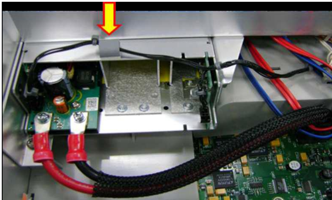
Bulk power supply cable and on/off cable routing
