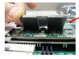
3. **Install new heat spreader:** Gently press the new heat spreader in place. There are no screws that hold the heat spreader on the board or guides for placement of the heat spreader. Simply match the placement of the heat spreader with the pictures below and gently press it in to place. The top cover will hold the heat spreader in place.
