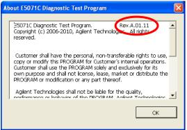
**Step-2:** Update the firmware to Rev. A.09.61 or above, then the Diagnostics Test is automatically updated to A.01.12 or above.
