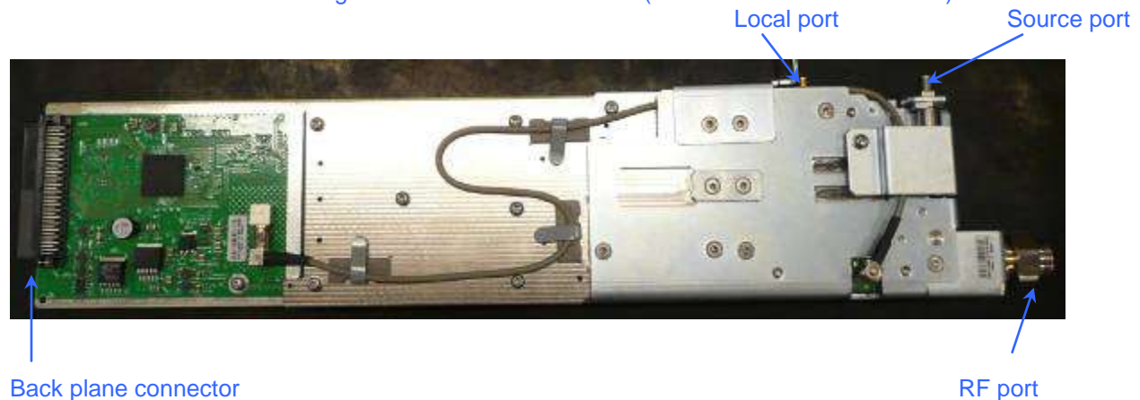
Fig 1. Bridge module port location
