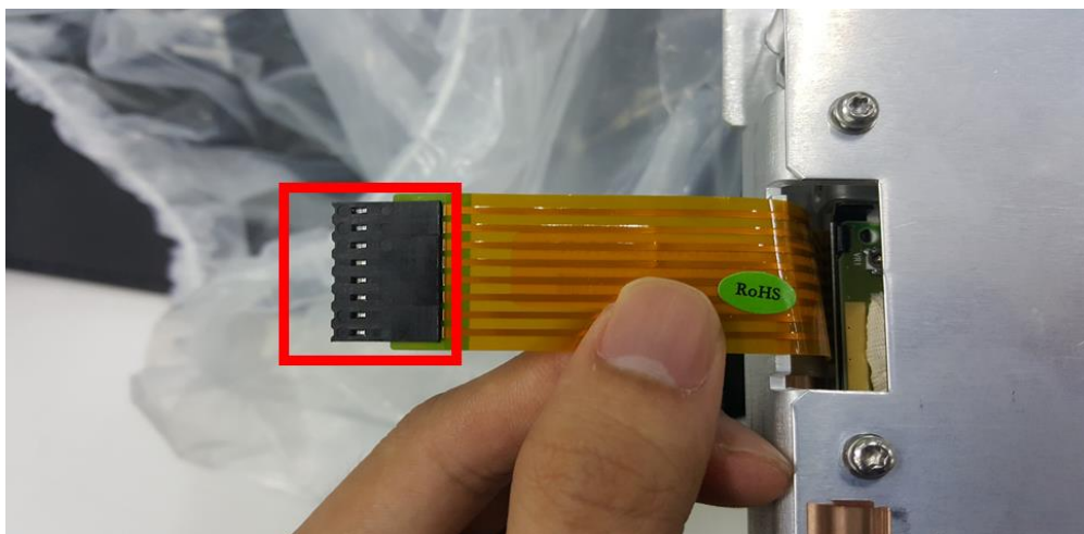
Figure 2 Touch Panel Cable's direction (The hole will be facing inward)
