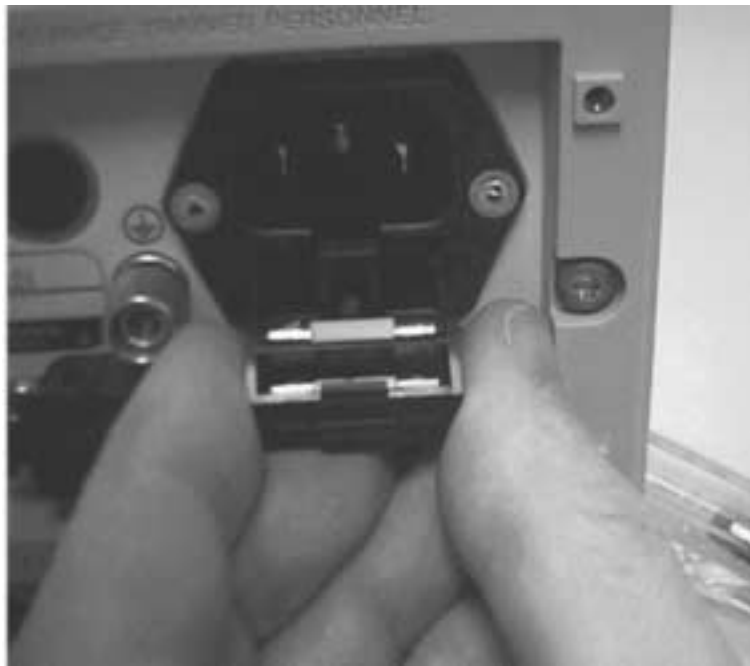
Figure 6. Replacing Fuse Holder
