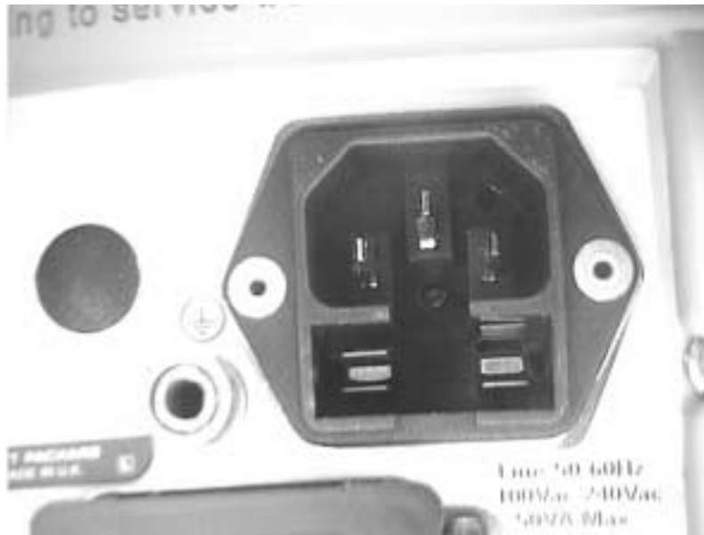
Figure 3. Fuse Clips That May be Damaged or Require Bending.
