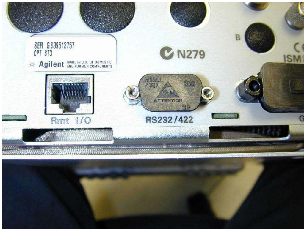
Figure 1. Example of a badly positioned gasket.
