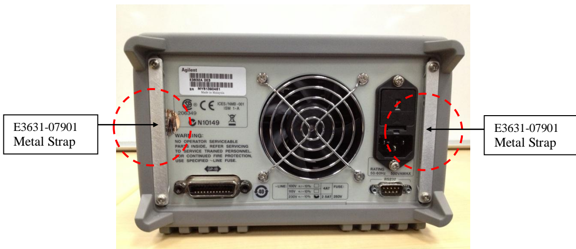
Figure 4: Secure with metal straps – no gap observed between the bumper and chassis
