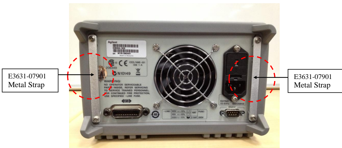
Figure 3: Secure with metal straps – no gap observed between the bumper and chassis
