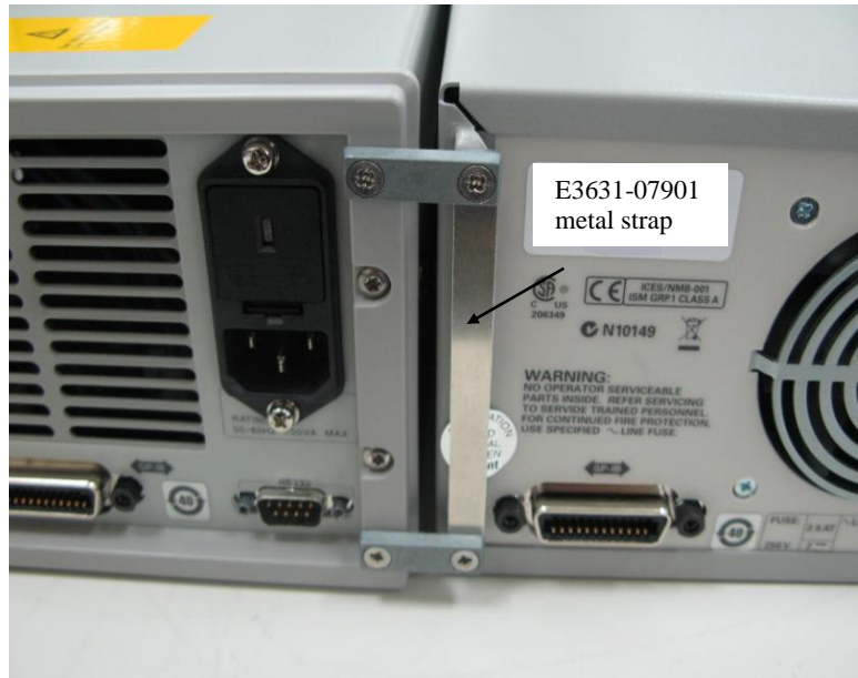
Figure 4: Rear view rear lock link secured with metal straps kit for side-by-side rack mounting
