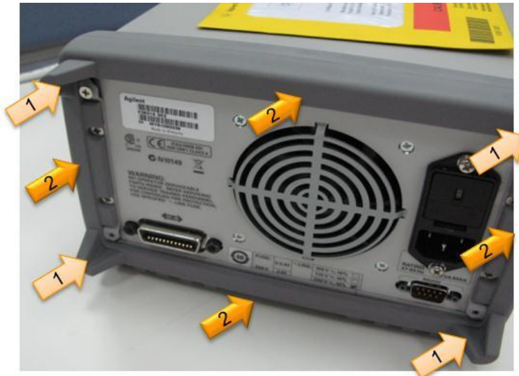
Figure 2: Proper fitting method for instrument rear bumper
