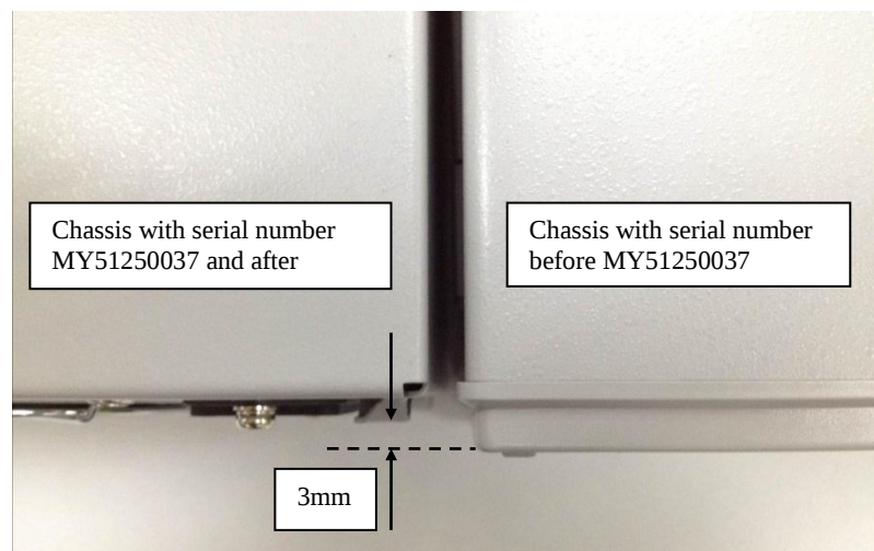
Figure 1: Top view 3mm gap observed between two different chassis designs
