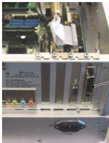
Figure 1, New GPIB Assembly Location
