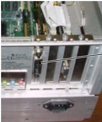
Figure 2, Original GPIB Assembly Location
