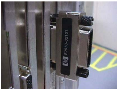
Figure 3, GPIB Extender Installed.
