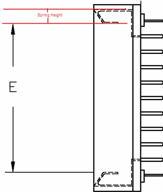
This design enhancement is intended to position the contact beams closer to the middle of the socket and increase the normal force exerted on the contacts of the chips mated to the socket.
