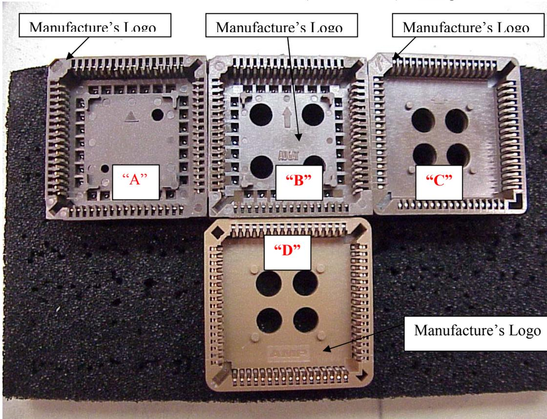
The following information will help identify each socket type and manufacturer. The manufacturer's logo can be identified as shown. After the **16-Bit MCU 16 MHZ 68PLCC CMOS IC** has been removed there are also mold markings that can be easily viewed these markings should be used to identify a **Good or Defective socket**.
