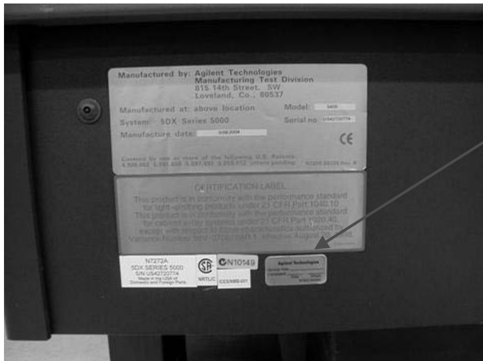
Figure 6: Detailed view of N7200-84366 service note label installed at lower right of label area
