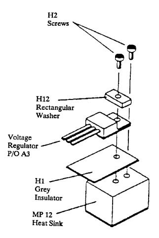
Figure 1. New Heatsink Mounting Arrangement
