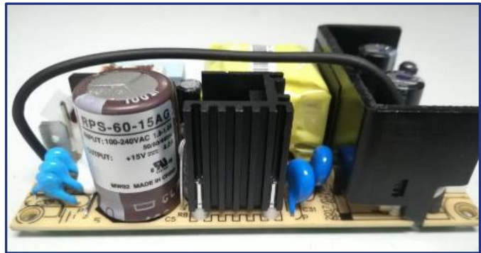
New MeanWell Power Supply (PN 0950-6082)
