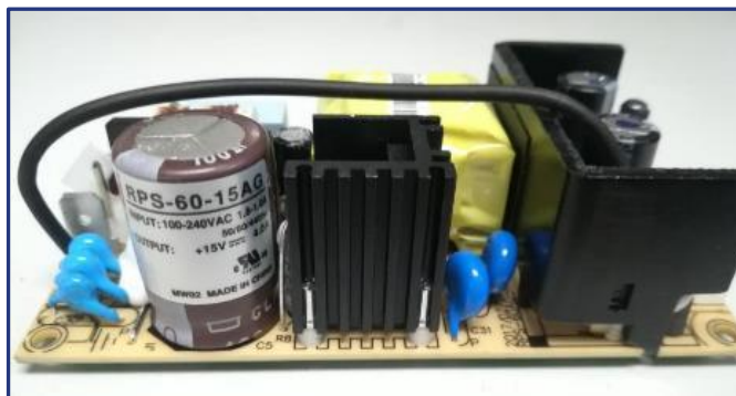
New MeanWell Power Supply (PN 0950-6082)
