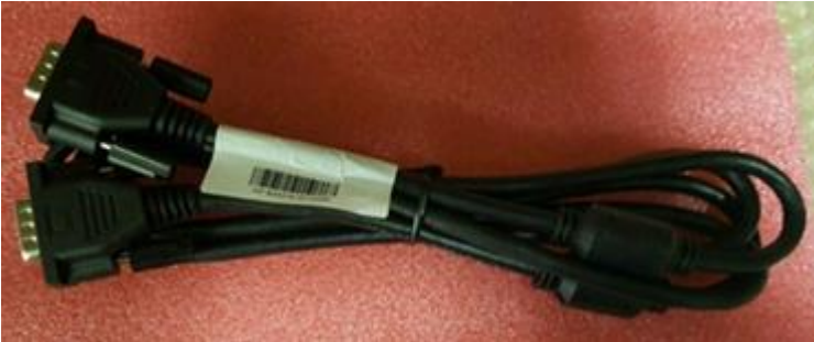
Figure 3a: new VGA cable KPN: 8121-3377
