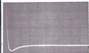
200 mV/cm, 1 msec/cm PULSE PERIOD (PP) = 60 msec SQW = 5.0V
