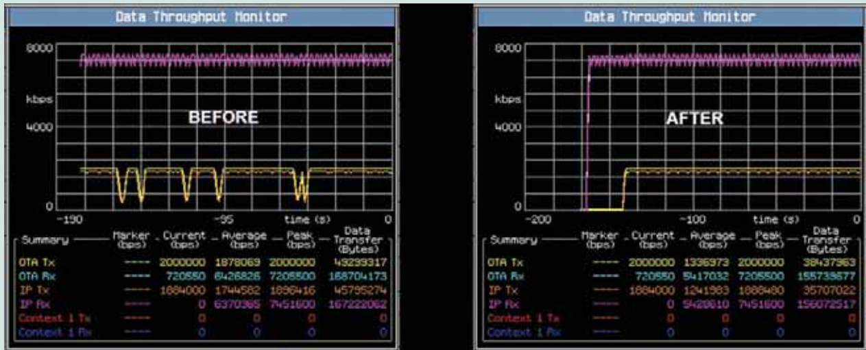
Figure 3. Data “drop outs” identified during physical layer integration
