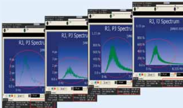
Figure 5. Increased memory size produced higher-resolution RJ, PJ spectra and larger RJ (rms) values
