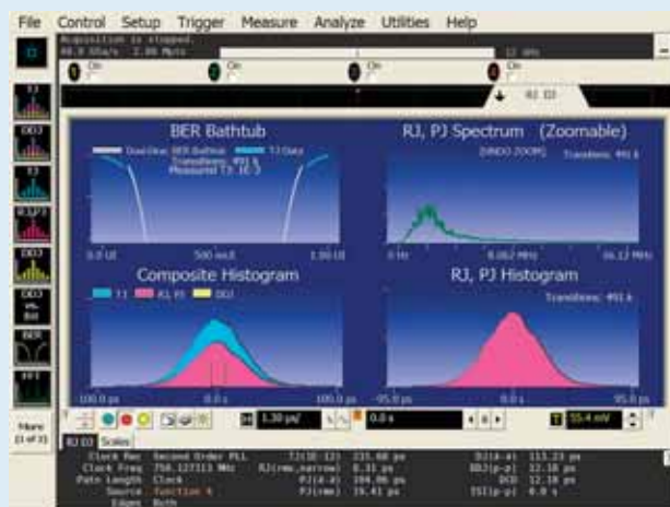
Figure 3. With memory size of 2 Mpts, TJ = 231.68 ps and RJ (rms) = 8.31 ps
