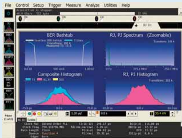
Figure 2. With memory size set to 512 Kpts, TJ = 148.17 ps and RJ (rms) = 2.26 ps
