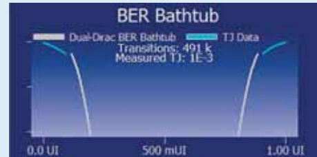
Figure 4. Breaks in the BER bathtub trace exist between the measured and extrapolated sections
