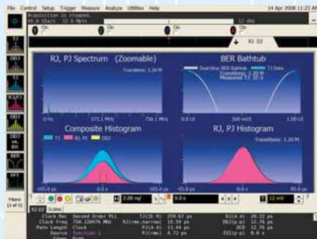
Figure 9. With memory size set to 32 Mpts, the EZJIT Plus software measured a TJ of 259.67 ps at a BER level of 10^{-9}
