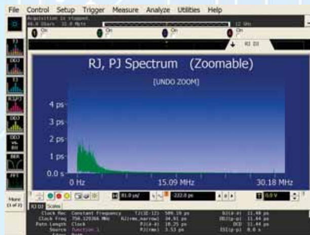
Figure 10. With constant-frequency CDR, the RJ, PJ spectrum exhibits a large flicker noise effect (TJ is 509.19 ps)
