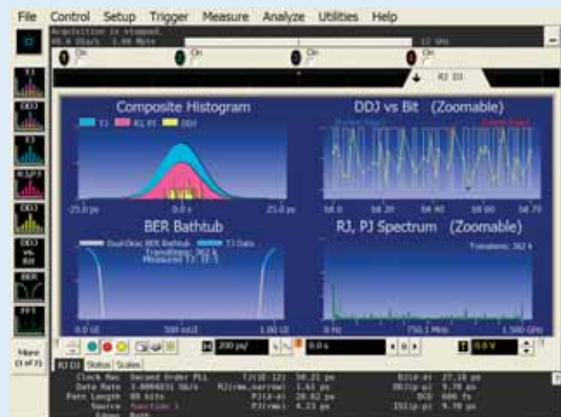
Figure 1. Four-window display includes composite histogram, data-dependent jitter (DDJ) versus bit, BER bathtub plot, and RJ, PJ spectrum
