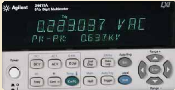
Figure 1. The Agilent 34411A measuring 223 V in the main display and 637 V pp in the lower display
