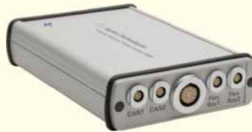
Figure 4. Agilent FlexRay VPT1000 supports protocol layer testing.
