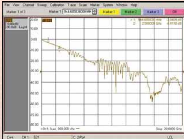
Figure 5. S_{21} of the 20-inch trace on a demo board
