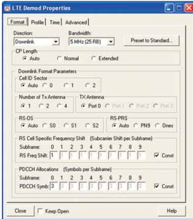
Figure 11. Example of a setup menu for downlink signal analysis
