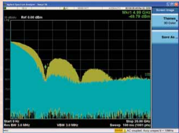
Figure 6. Data signal spectrum before (yellow) and after (blue) propagating through the demo board
