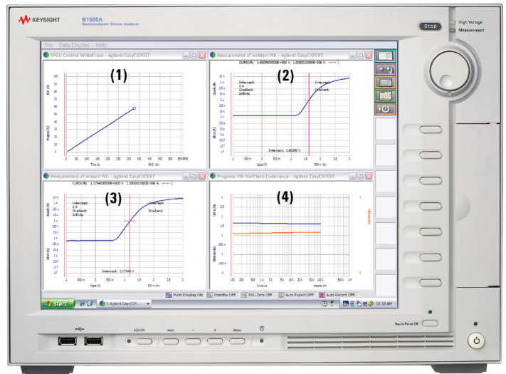
Figure 7. Snapshot of B1500A write/erase endurance testing
