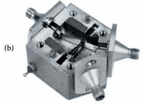
Figure 1. The "edge-line" transmission line concept (a) uses a flat center-conductor perpendicular to two ground planes which concentrates the field pattern at its edges. This allows a flexible "flipper" blade in the HP 8761A/B Coaxial Switch (b) to contact either output connector port.
