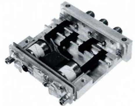
Figure 2. Internal view of HP 33311B Switch shows "see-saw" action of shorting bar plungers. Note the two internal 50-ohm terminations on sapphire at the edges.
