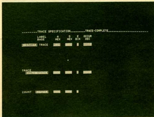
Figure 13. Trace Specification to Qualify the Logic Analyzer to only Capture Memory Write Transactions.
