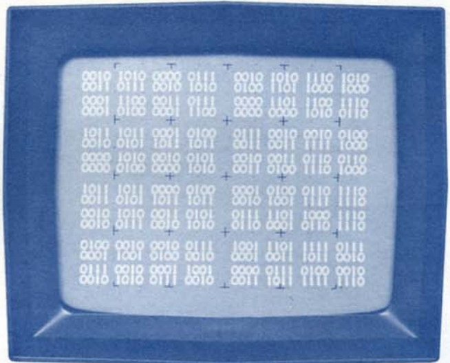
1. A functional display of ONEs and ZEROs gives designers an overview of the operation of a digital system. Words are captured in the analyzer's memory.
