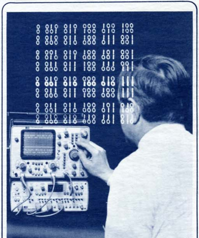
Figure 7. The 1740S system consisting of a 1607A logic state analyzer and a specially modified 1740A oscilloscope was created in response to the need to combine both time and data domain measurement capability in a convenient form.
