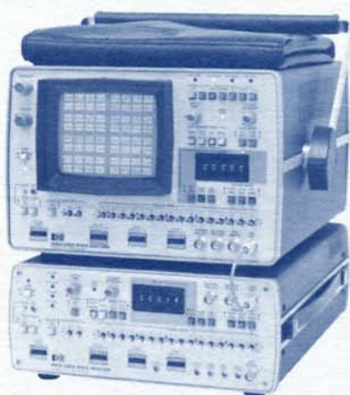
Figure 4. A 1600S system consists of two logic analyzers, the 1600A and the 1607A, connected together to form one 32-bit analyzer capable of simultaneously displaying and triggering on two independently operating 16-bit data streams. It can easily capture and display simultaneously address and data up to 32-bits in width, show data being read from the same bus at two different threshold settings and Exclusive-OR the display to highlight differences, and show dual-clock systems on one screen for real time analysis of such things as I/O data transfer.
