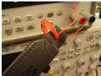
Figure 3. Improve the probe sensitivity by winding several turns of the conductor under test around the probe.
