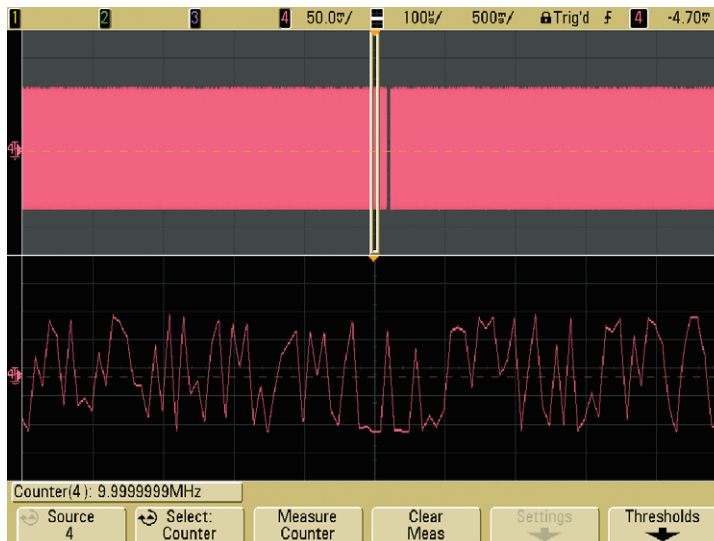
Figure 2. If an external 10-MHz reference is used, the counter is as accurate as the externally fed 10-MHz signal and the measurement resolution is increased to up to 8 digits.
