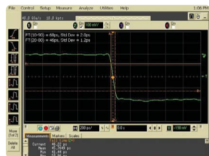
B. Real-time scope, 10 GHz bandwidth. Fall time measurement 46 ps.
