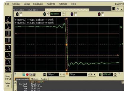
B. Real-time scope, 10 GHz bandwidth. Fall time measurement 30 ps.
