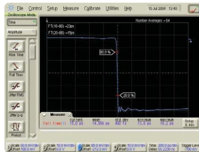
A. Sequential sampling scope, 50 GHz bandwidth. Fall time measurement 15 ps.
