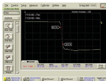
A. Sequential sampling scope, 50 GHz bandwidth. Fall time measurement 46 ps.
