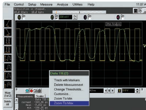
Figure 9. The Zoom to Max and Zoom to Min functions on the Agilent serial data analysis package allow you to jump to the signal edge with the worst-case jitter.
