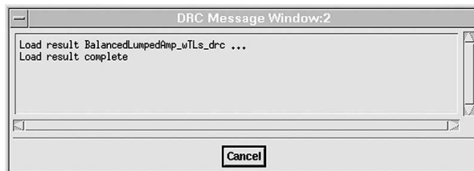
Figure B-4. Message that appears after the DRC results have been loaded.
