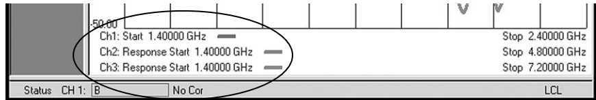
Figure 5. The frequency range indicates whether the analyzer is operating in standard mode or frequency-offset mode.
