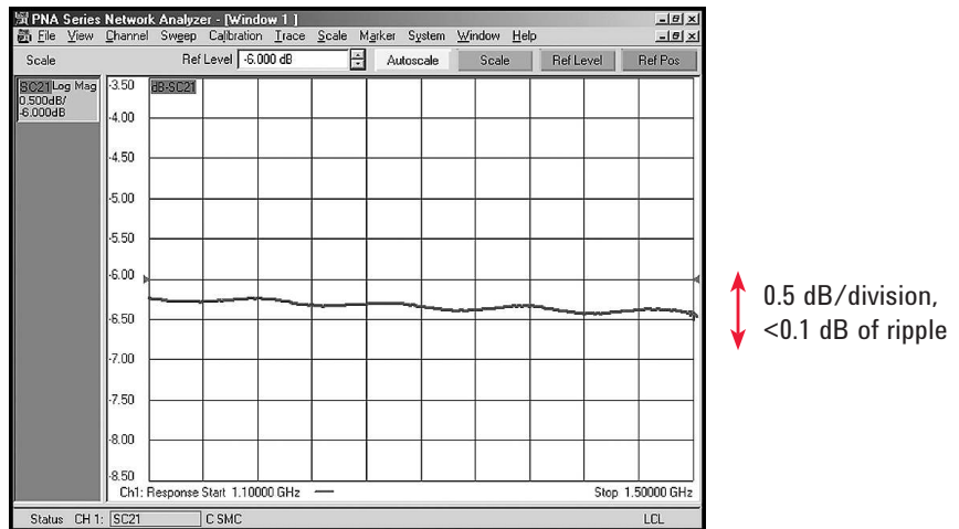
Figure 28. Conversion loss (SC21) measurement with 6 dB of input attenuation – showing little ripple.
