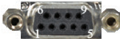
Figure 5. Power I/O connector on rear panel of PNA-X.
