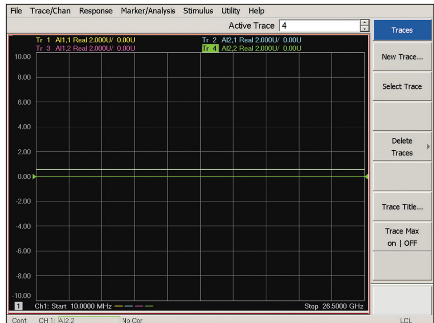
Figure 9. AI1 and AI2 traces displayed on the PNA-X, and with different source ports.
