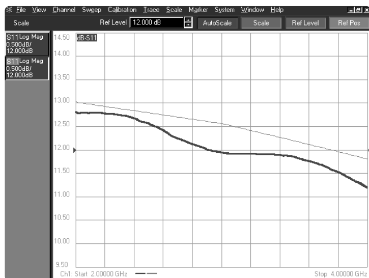
Figure 21. Measured S21 of a surface mount amplifier. The lower trace shows the response using a standard coaxial calibration and the upper trace shows the de-embedded response
