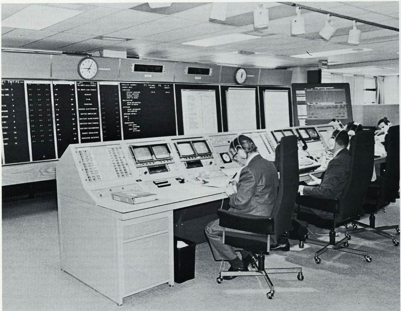
Figure 4. The Operations Room at the Satellite Control Centre. Here, all satellite measurement parameters are displayed and operations personnel initiate control and command signals to the satellite.
