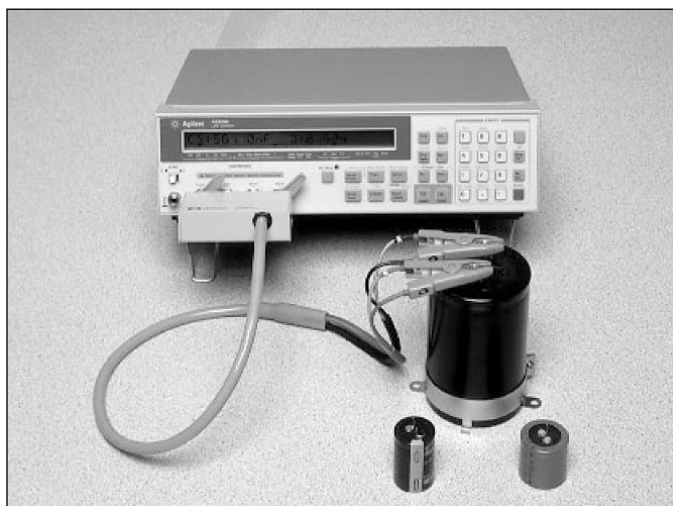
Figure 3. Big Electrodes Electrolytic Capacitors Measurement using the Agilent 16089A
