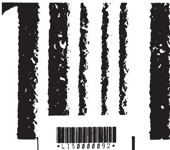
14c. Poor Print Quality (Poorly Inked Ribbon)
