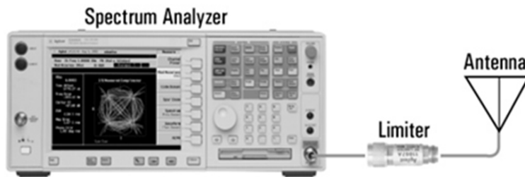
FIGURE 2: Shown here is a typical application using a power limiter to protect an RF instrument. In this case, the input of a spectrum analyzer is protected from an inadvertent overload due to high-level signals from an antenna.
