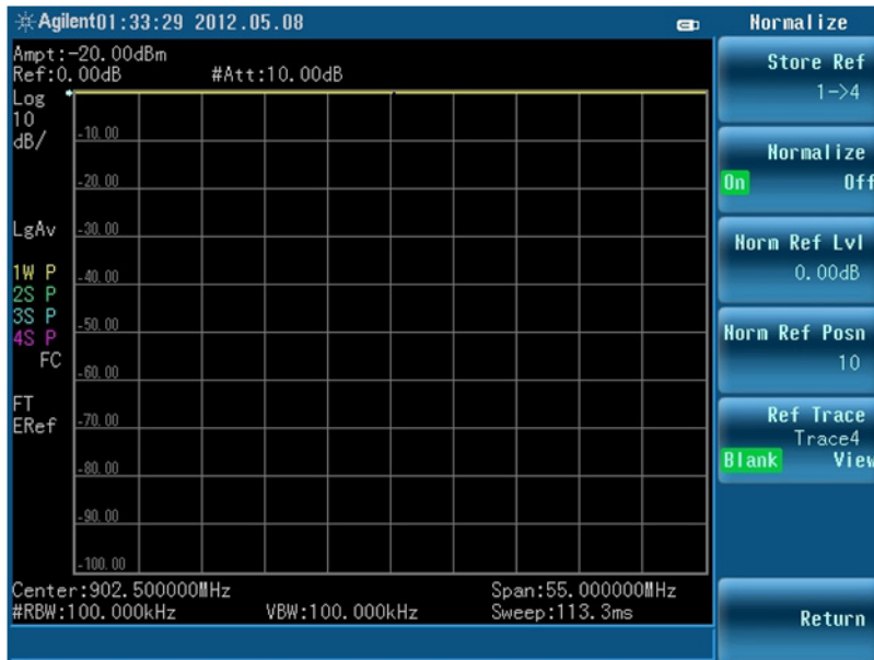
Figure 6. Normalization establishes a 0-dB reference trace
