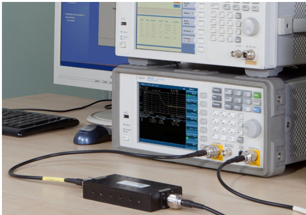
Figure 4. Transmission measurement setup
